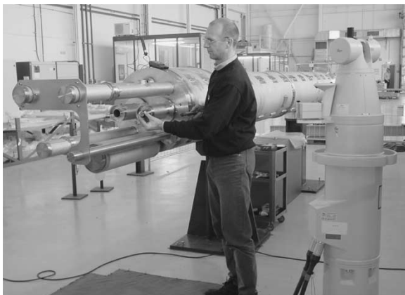
Fig. 3. Mechanical measurement of coil mass with laser tracker system.
